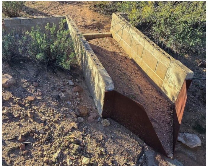
The device found at the study site was soon identified as a Parshall flume – a standardized device hydrologists use to measure volumetric water flow.
